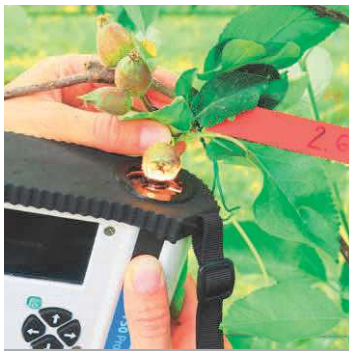
Fruit drop prediction based on spectral VISNIR scanning at the research sites KOB (D) and Laimburg Research Centre (I) VZ Laimburg
