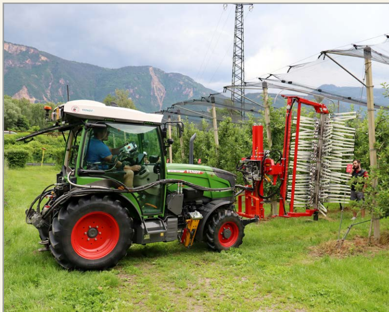
The Laimburg Research Centre presented the initial results of thinning with a fruit thinning machine.
