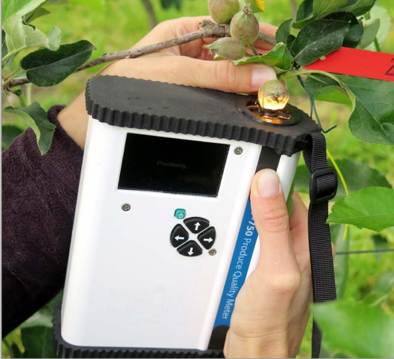
Device for fruit fall prediction based on VIS/NIR scanning
